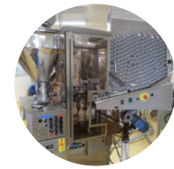
1 tubes conditionning line
